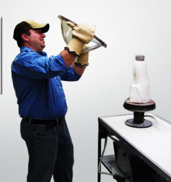
Take to model, flip like normal blister forming, pull down with a slight twisting motion and apply vacuum.
