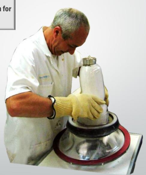
Take a flat head screw driver and place between aluminum support and plastic and create a void. This will allow you to easily separate the plastic from the aluminum ring support when the plastic has cooled.
