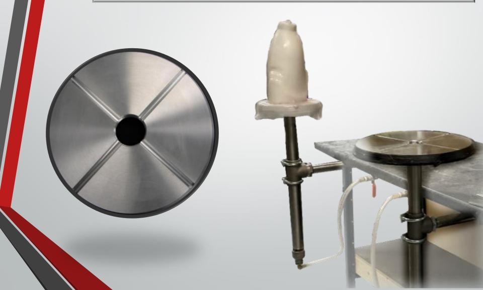
Place Ringmaster® sheet on the aluminum support ring with the spru facing downward.
