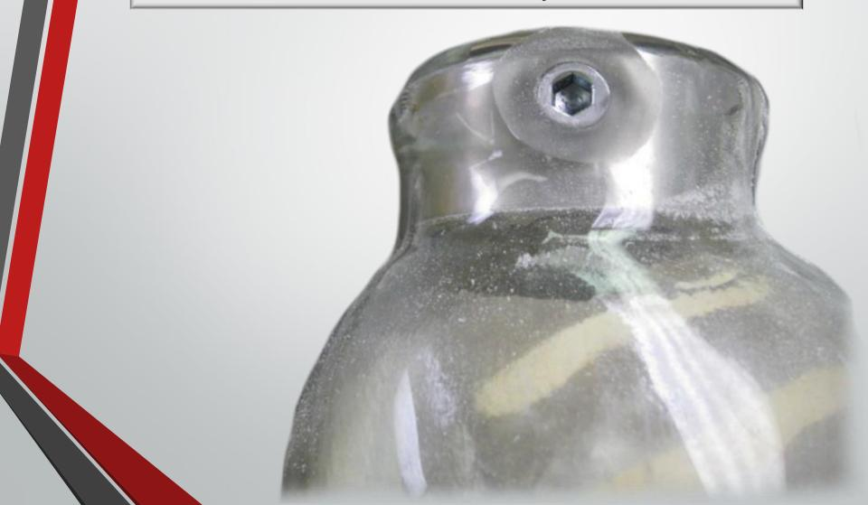
The thermoforming dummy makes it easy to drill out the holes. The thermoforming set screws that were positioned slightly raised gives distinct points for the four hole pattern. No guessing!
