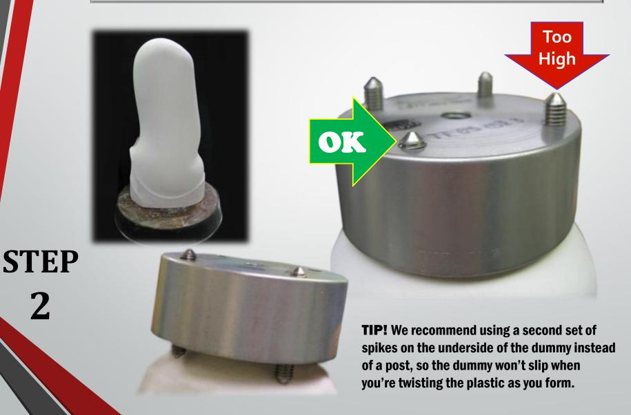
A brand new item that can also be used is the removable center spike <u>TF-RCS</u>. You can take the center spike and drill in into the center of model and then screw the dummy right onto the top
